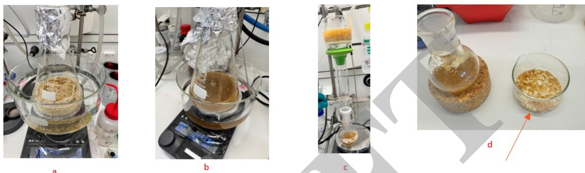
Figure 19: Strating washed CF + 2% NaOH after 5h (a), CF + 2% NaOH after 34h (b), filtration of neutralized hydrolysate (c), freeze-dried and residual hydrolysate (d)
