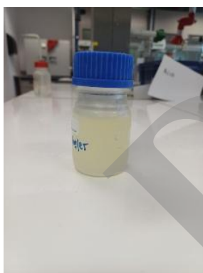
Figure 9: Alkyl ester of microbial oil: colorless/translucent sample sent for application testing
