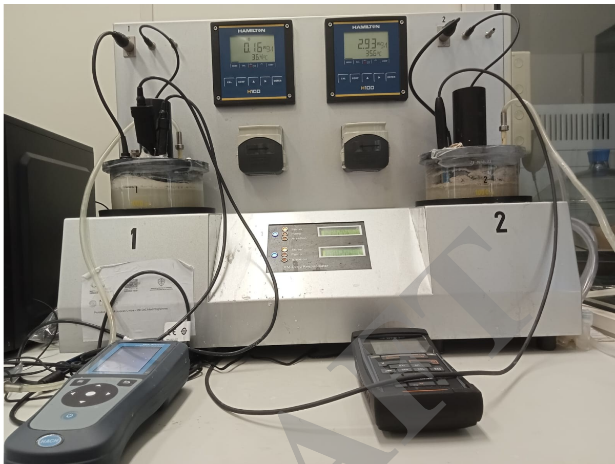
Figure 1. Laboratory-scale anaerobic fermentation setup.
